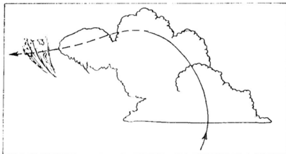
Figure 2.17 Schematic representation of the generation of rain in a cumulus. The line through the model cloud represents an idealized (smoothed) trajectory of air through the cloud; it is drawn continuously through the regions of strong updrafts and greatest concentrations of condensed water, and dashed where evaporation is dominant (after Ludlam, 1980).
