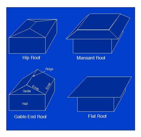
Figure A2.1. Illustration of roof terminology
