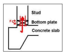
**Figure 4.** Typical wall cross section on concrete slab foundation showing a bottom plate bolted to the foundation and straight-nailed into the wall stud. Connections and failure points ("F") are in red.
