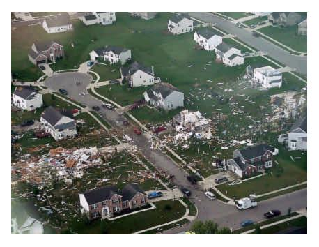
**Figure 11.** Path of a tornado in Xenia, OH, on 20 September 2000, showing near total destruction of one home (lower left) even as nearby homes have suffered virtually no structural damage. This is unlikely to be the result of extreme winds but is more likely to be a structural failure associated with that particular home, and is complicated by the damage to the home across the street, which surely produced many projectiles. (Photograph courtesy of J.H. Golden, used by permission).
