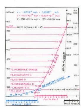
**Figure 1.** Illustration of the relationship of the Fujita scale as a connection between the Beaufort and Mach scales (Fujita 1987).
