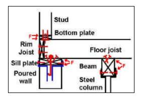
**Figure 11.** Typical cross section of a poured concrete wall foundation showing miled and bolted connections with failure points (in red) and strapped connections (in blue). Center beam is wood or steel.
