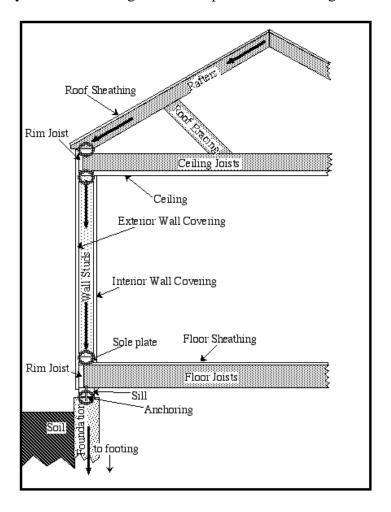
**Figure 8.** Schematic illustration of the load path for a single-story, wood-frame home, with arrows showing the transfer of the gravity load from the roof to the ground. Circles indicate locations for securing attachments (see BPAT [1999] for details).
