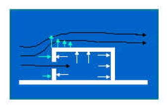
**Figure 10.** Schematic illustration of "pressurization" as impinging wind (black) enters through a puncture of a building's envelope, and the resulting pressure forces from both interior pressurization (white) and exterior airflow (turquoise).
