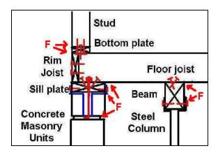
**Figure 14.** Typical cross section of a masonry wall foundation showing nailed and bolted connections (in red) and strapped connections (in blue). Center beam is wood or steel. Failure of this foundation type frequently occurs at areas denoted by the letter "F".
