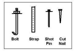
**Figure 1.** Common types of foundation fasteners.
