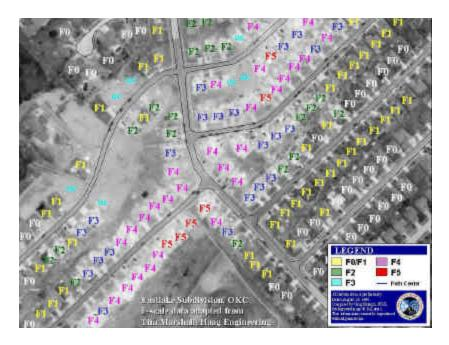
**Figure 42.** Example of detailed street map, showing home locations and F-scale estimates (Image courtesy of the National Severe Storms Laboratory).
