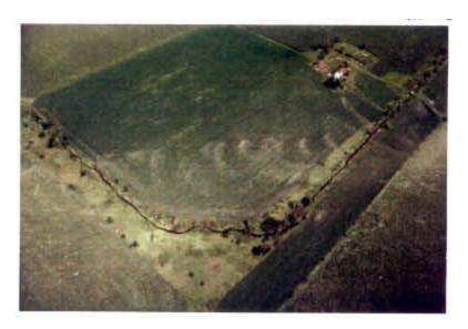
Figure 15. Example of cycloidal debris marks associated with a multip le-vortex tornado (Fujita 1992).
