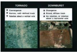
Figure 44. Illustration of the difference between tornado (left) and downburst (debris) damage from the air.
