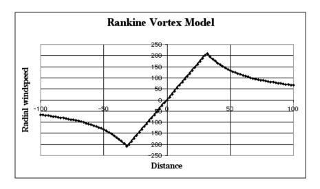
**Figure 6.** Radial wind profile in an idealized Rankine Combined Vortex Model, having a *radius of maximum winds* at a distance of about 30 units from the axis. Speed and distance units are arbitrary.
