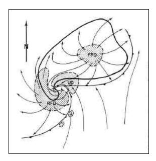
**Figure 21.** Basic airflow associated with a supercell storm (after Lemon and Doswell 1979), showing the forward and rear flank downdrafts, denoted "FFD" and "RFD" respectively. The updraft is indicated by fined stippling and labeled "UD" – the possible location of a tornado is indicated by the circled "T" symbol.
