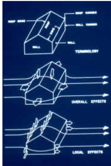
**Figure 9.** Schematic illustration of airflow interacting with a structure, showing the resulting pressure effects. The “local” effects arise because the increased airflow at corners due to the Bernoulli effect.
