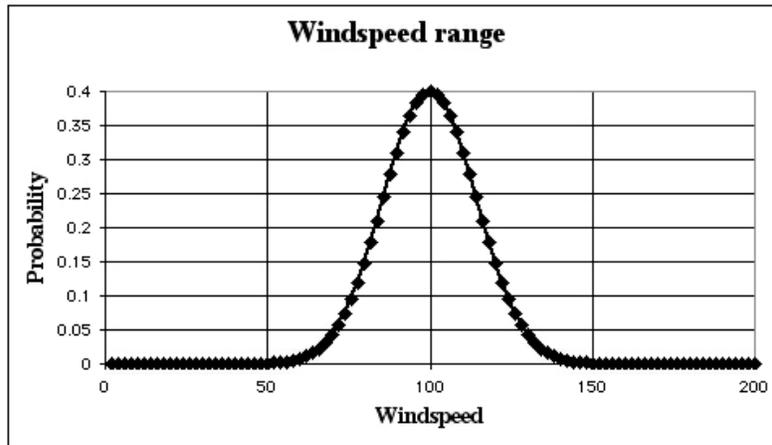
**Figure 5.** Schematic illustration of the probability that a particular damage event was produced by wind of a given value – the total area under the curve has a probability of 1.0. This distribution is symmetric about the most probable value and has only one peak probability, but in *real* examples, the distribution might not be so simple.
