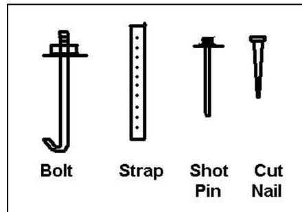
**Figure 1.** Common types of foundation fasteners.
