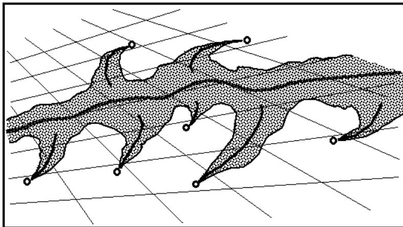
**Figure 12.** Schematic illustration how damage produced by the failure of a weak structure can create “damage cones” on the periphery of a tornado track (cf. Fig. 3) – from Speheger et al. (2002).
