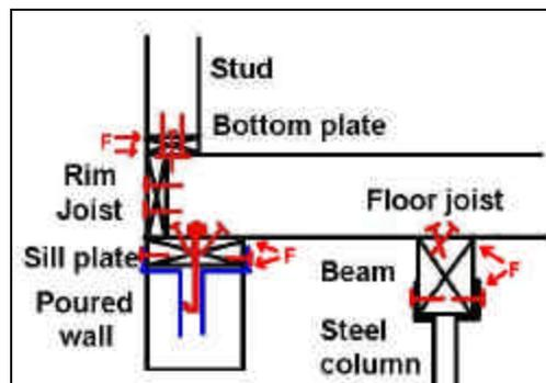
**Figure 11.** Typical cross section of a poured concrete wall foundation showing nailed and bolted connections with failure points (in red) and strapped connections (in blue). Center beam is wood or steel.
