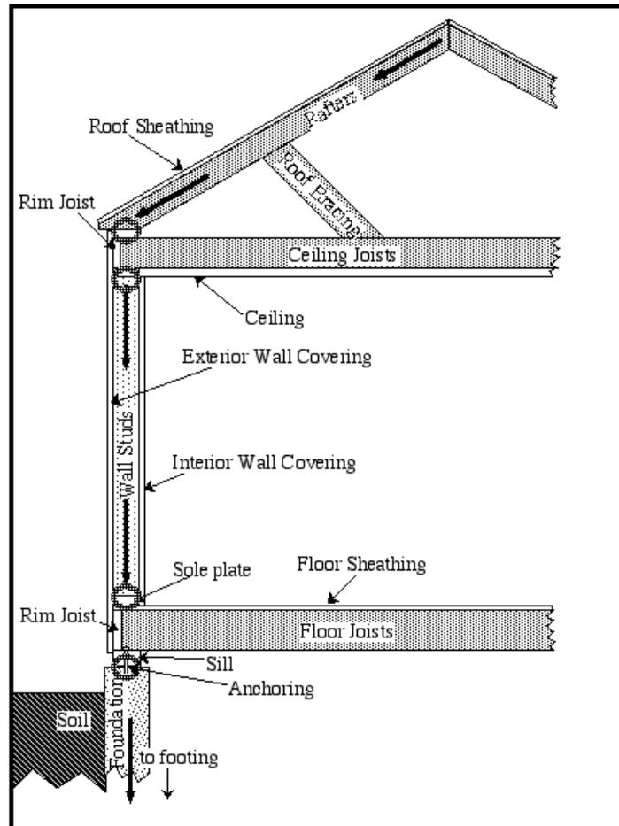
**Figure 8.** Schematic illustration of the load path for a single-story, wood-frame home, with arrows showing the transfer of the gravity load from the roof to the ground. Circles indicate locations for securing attachments (see BPAT [1999] for details).
