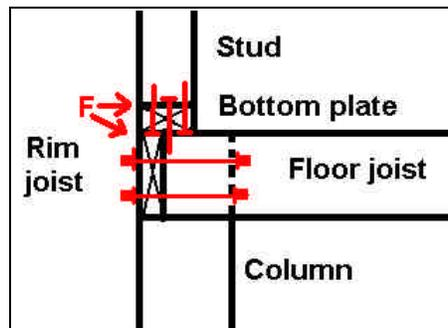
**Figure 17.** Typical cross section of home elevated on timber piles, concrete or masonry columns. Floors are usually bolted or strapped to the columns (in red). Common failure points are the nailed connections where the wall is attached to the floor.
