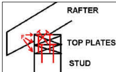
**Figure 22.** Typical cross section of roof/wall top plate showing nailed connections and common failure points (in red).
