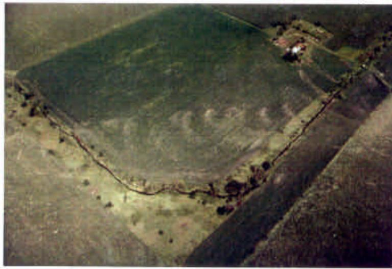
**Figure 15.** Example of cycloidal debris marks associated with a multiple-vortex tornado (Fujita 1992).
