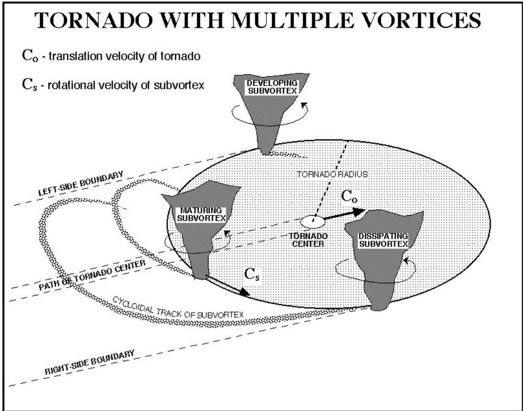
**Figure 16.** Schematic model of a tornado with multiple subvortices (adapted from Fujita 1971).
