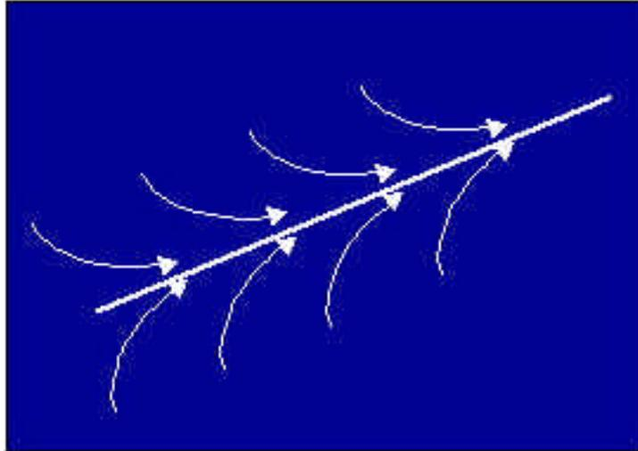
**Figure 33.** Schematic illustration of the near-surface flow directions produced by a moving, relatively long-lived source of convergence, such as a single-vortex tornado. When the tornado is moving rapidly, the centerline might be shifted toward the left of the track.
