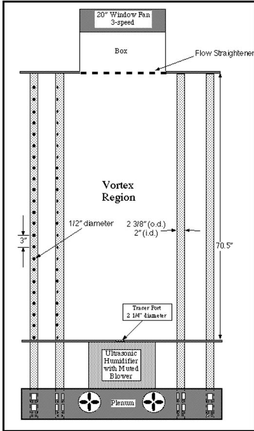
Fig. 2. Schematic view of simulator, with the vertical tubes at the front omitted for clarity (see Fig. 3). Horizontal airflow exits from the vertical tubes; this flow comes from fans (at the bottom) pushing air into a box, so that air is forced upward through the tubes. The ultrasonic humidifier produces a fine mist for flow visualization. The large fan at the top produces inflow within the vortex chamber.
