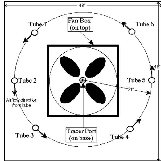
Fig. 3. View of the simulator from above, showing all six of the vertical tube locations and the tangential flow produced by the tubes.
