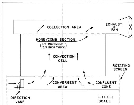
Fig. 1. Schematic diagram of a Ward-type vortex simulation chamber, showing the main components as first developed by Ward.
