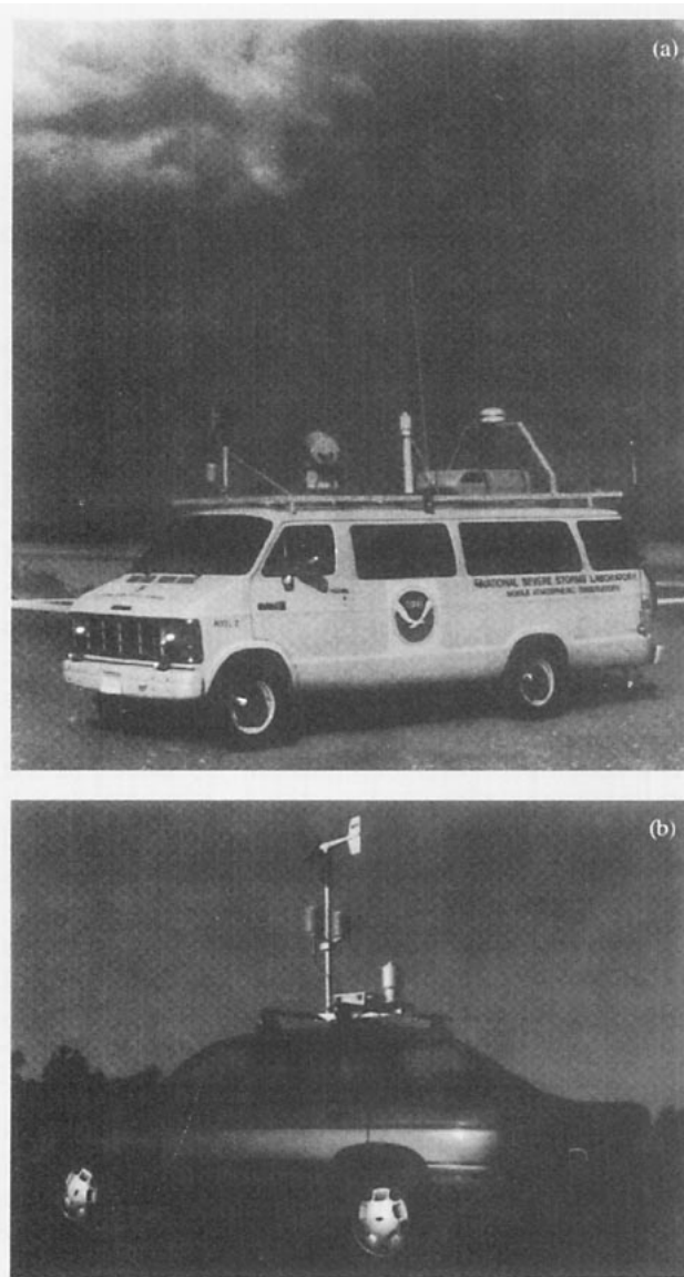
FIG. 5. (a) An NSSL mobile laboratory, and (b) car outfitted with prototype mobile mesonet equipment. Temperature, humidity, and wind sensors are on the short mast mounted atop the roof rack.
